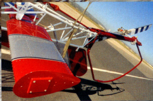
The horizontally opposed, six-cylinder Lycoming engine (above) is mounted vertically and is exposed to the elements. A synchronized (with the cyclic) elevator (right) assists in pitch control.
