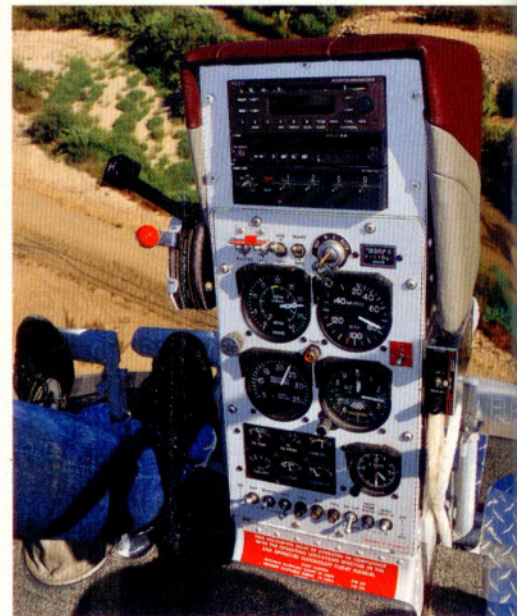
The right pilot's collective/throttle (left) peeks out from between the seats. The instrument pedestal (below) has room for only the basics and is modified to be shorter than when it left the factory.
